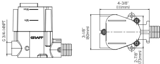
**G-8077** *Concealed cut-off valve module - rough*
