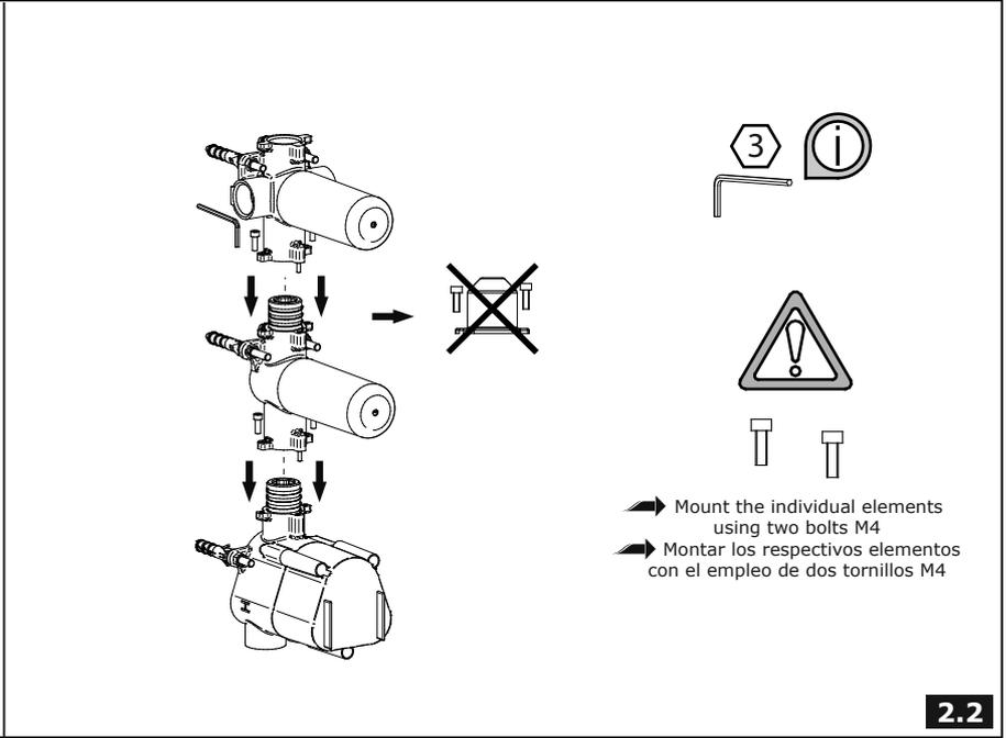
➔ Mount the individual elements using two bolts M4
