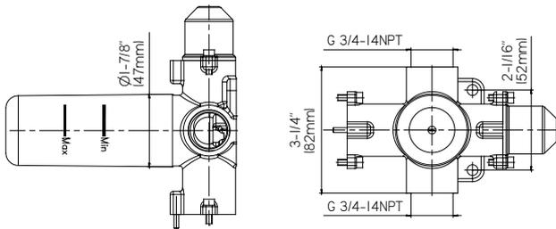
**G-8053S** *Concealed 3-way diverter module without OFF function - rough*
