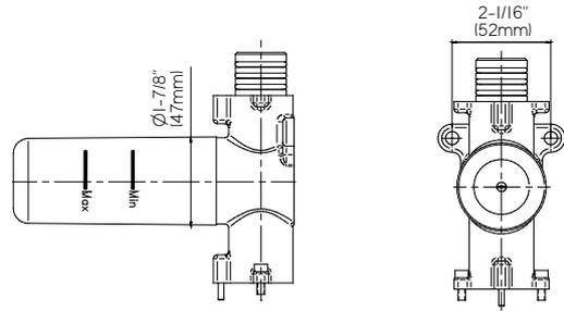
**G-8052S** *Concealed 2-way diverter module without OFF function - rough*
